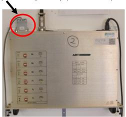
2. Adjust amp gain settings to 1000 (i.e. set all switches to 'close' on all channels).
